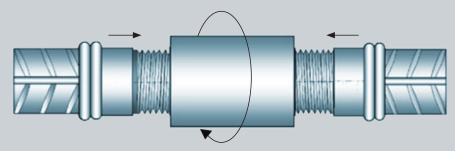
3 Finished joint tightened with a torque wrench until no further movement and torque requirements of table 2 are met
