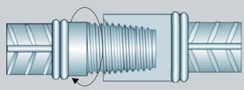
2 The joint is then screwed together using a wrench
